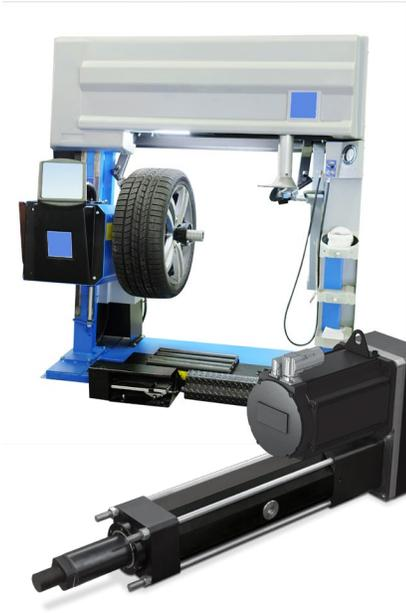
*An OEM tire inspection process had used a press machine with a set of hydraulic actuators and back springs that brought two rim halves into position. The tire is then inflated and tested under pressure. Tolomatic's RSX096 rod-style extreme force electric actuators were selected to replace the hydraulic cylinders resulting in higher energy efficiency, reduced ambient noise, elimination of frequent hydraulic maintenance and fluid leaks, and significant savings in floor space.*
