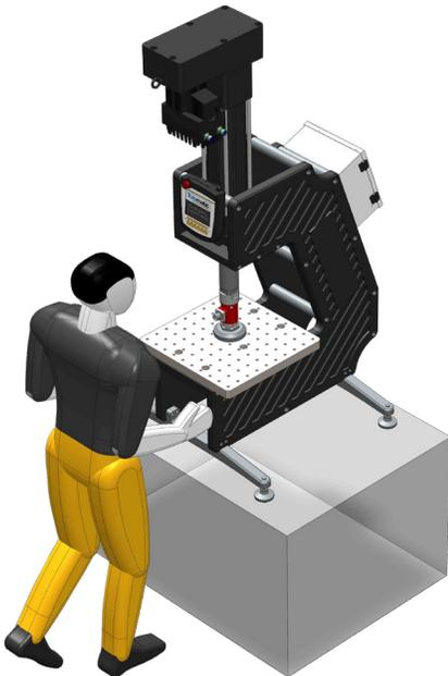
*Electric linear actuators are more efficient and offer increased precision compared to hydraulic cylinders, making this technology ideal for press applications that require accuracy, speed and flexibility along with vastly reduced maintenance.*
