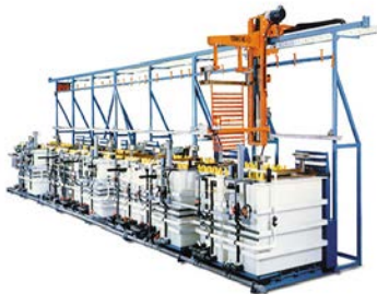
A multi-axis gantry is often the ideal solution for manufacturing processes that requires a combination of material handling and precision through a multi-step process, such as this dip tank application for plating
