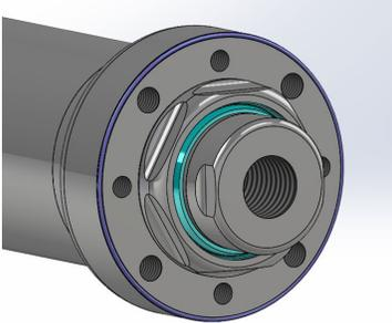
Figure 3.2: RSH Standard front face mounting holes
