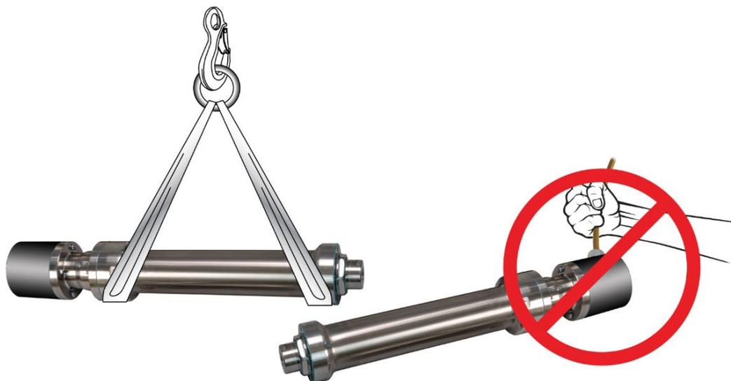
Figure 4.1: Proper (and improper) RSH Lifting Technique
