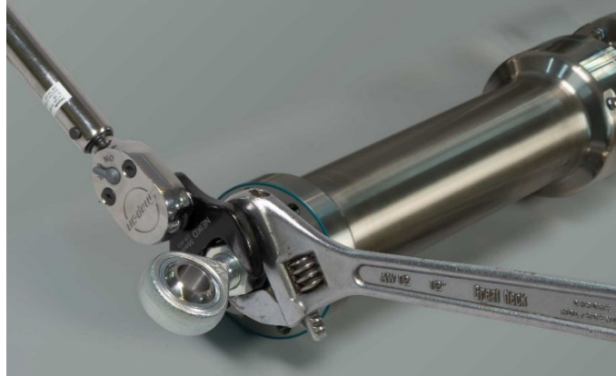
Figure 4.3: For RSH hold the thrust rod stationary using a wrench on the flats at the end of the thrust rod when attaching accessories, linkages or load to the actuator.
