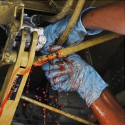
It's not a matter of *if* but *when* hydraulic systems will leak or break. Clean-up is messy and time-consuming. When hydraulics fail, the production parts/product may need to be scrapped out and production stopped while repairs and cleanup are undertaken.
