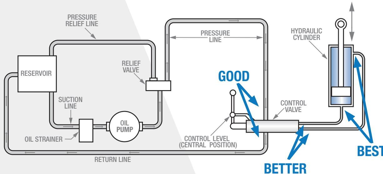
The next best and most practical way is to measure hydraulic pressures in the cylinder while the process is in operation.
