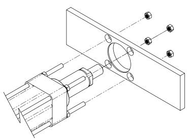
Figure 3-8 RSX extended tie rods option
