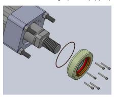
Figure 6-1 RSX seal cartridge exploded view
