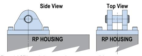
Figure 4-9 RSX rear clevis mount option on reverse parallel motor mount actuator
