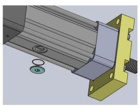
Figure 6-2 RSX lubrication access cover exploded view
