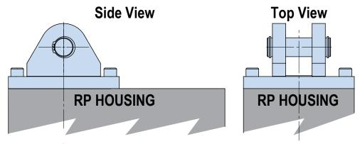
Figure 3-4 RSX rear clevis mount option on reverse parallel motor mount actuator
