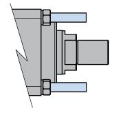
Figure 4-10 RSX extended tie rod mount option
