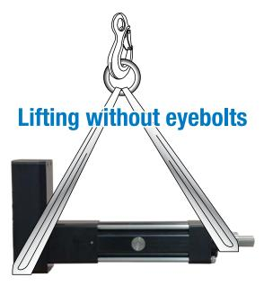
Figure 4-2 Lift RSX properly without eyebolts
