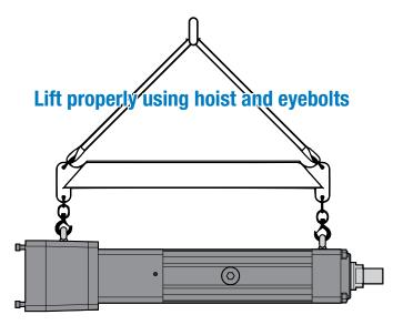
Figure 4-1 Lift RSX properly using hoist and eyebolts
