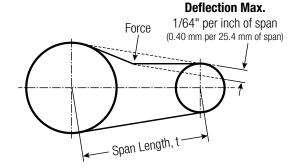
Figure 4-4 RSX belt pulley diagram
