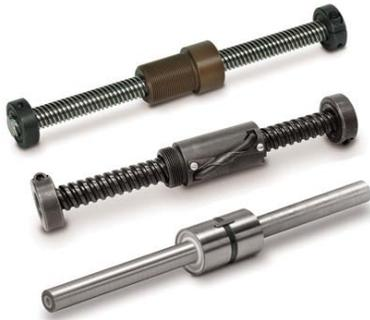
**Acme/Trapezoidal Screw with Bronze Nut** – Quiet, inefficient, and cost effective. These screws are well suited for applications that do not require high or continuous duty cycles. By design their low efficiency ratings (<40%) allow them to be self-locking and also general resilient to shock loads and vibration. In general these screws are best utilized for duty a duty cycle of 40% or less.
