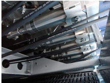
The low-maintenance features of the Tolomatic ERD actuators are important in this application due to the tight mounting quarters.
