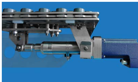
As the Tolomatic ERD actuator moves in and out, it activates the center plate above that rotates the cams on the top plate. These cams, in turn, activate rollers in the moving belt to create lateral movement.
