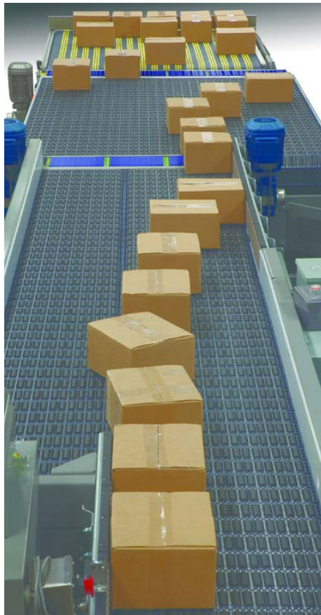
Tolomatic ERD electric actuators are used to organize pallet layers in the Intralox ARB™ alignment conveyor system.
