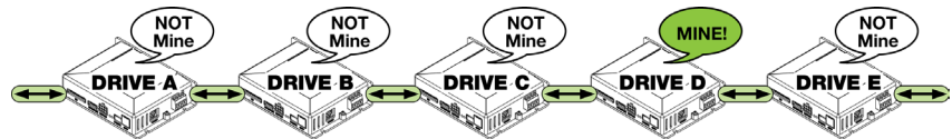
Figure 5: Packet flow through the daisy chain affects communication speeds as the drives determine whether the information being sent should be forwarded or processed.
