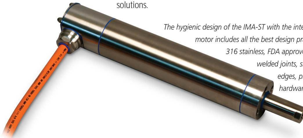
*The hygienic design of the IMA-ST with the integrated servo motor includes all the best design practices such as 316 stainless, FDA approved seals / o-rings, welded joints, smooth rounded edges, proper mounting hardware and an IP69k ingress protection rating.*
