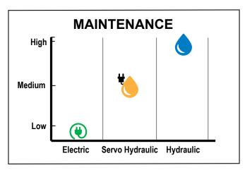
Figure 7: Electric systems require little or no maintenance compared to hydraulic systems.
