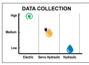
Figure 8: Electric systems provide the most data collection capabilities over servo hydraulic and conventional hydraulic systems.
