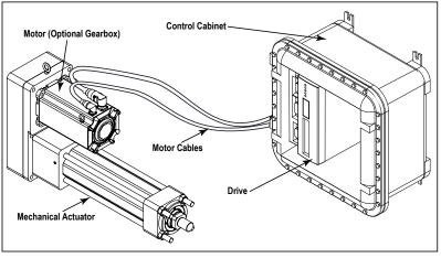
Figure 4: Electric system components
