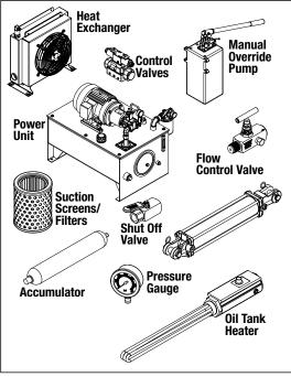
Figure 3: Hydraulic system components
