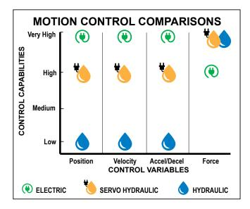
Figure 1: Control over all aspects of motion can be extremely important in critical applications where precise position, speed and force come into play. This chart shows the control capabilities of the three technologies.
