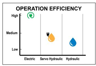
Figure 9: Compared to servo hydraulic and conventional hydraulic systems, electric systems operated far more efficiently.
