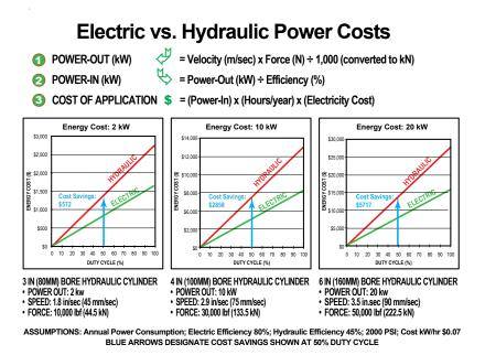
Figure 10: The above charts show the difference in electric utility costs for a hydraulic and an electric cylinder. The blue arrow depicts cylinder operation at 50% duty cycle and the resulting estimated utility costs. By dividing the efficiencies of the two technologies into one another, an approximate factor can be determined on electric utility cost based on when the actuators/cylinders are actually moving.
