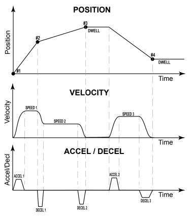
Figure 2: This chart shows different motion profile positions at different velocities with different accel/decel rates, all under full and precise control.
