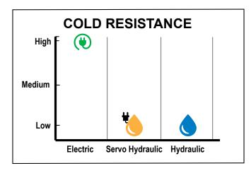
Figure 6: Electric systems are not susceptible to fluid thickening in cold temperatures and perform consistently despite fluctuations in temperature swings.
