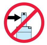
Figure 12: Side loading of rod actuators is not recommended because it places stress on
