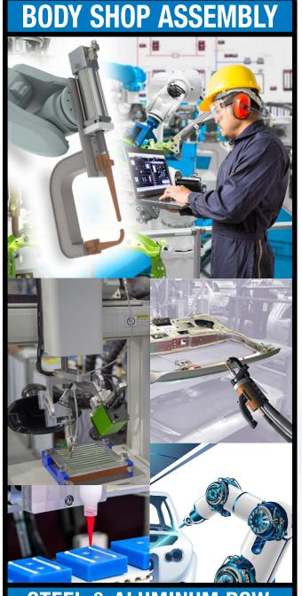
STEEL & ALUMINUM RSW, PNEUMATIC CLAMPING, PEDESTAL WELDING, PROJECTION WELDING, ADHESIVE DISPENSING, CLINCHING, HEMMING
