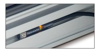
MX, RSA, GSA, and RSX products offer a large number of sensing choices. There are 12 switch choices: reed, solid state PNP (sourcing) or solid state NPN (sinking); in normally open or normally closed; with flying leads or quick-disconnnects.
