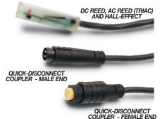
There are 10 sensing choices: DC reed, form A (open) or form C (open or closed); AC reed (Triac, open); Hall-effect, sourcing, PNP (open); Hall-effect, sinking, NPN (open); each with either flying leads or QD (quick disconnect).
