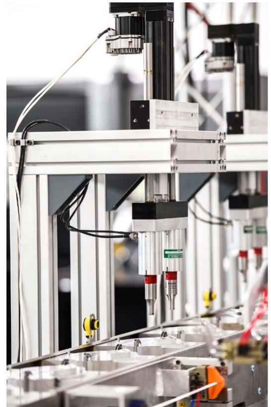
*Tolomatic GSA actuators (positioned above masks) provide motion function to apply elastic ear straps. Photo: Tolomatic, Inc.*
