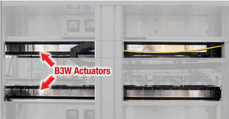
*Tolomatic B3W actuators (horizontal actuators, in red boxes, top and bottom of mask former) both move the material and support the heated form press. The unit is sealed to prevent contamination from particulate. Photo: Tolomatic, Inc.*
