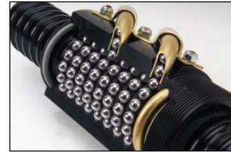
Capable of handling moderate loads, ball screw nut assemblies contain multiple ball bearings that cannot be made below a minimum size. When compared to a roller screw of similar size and lead, the ball bearings' radius requires a coarser pitch resulting in fewer points of contact. Combined with the smaller contact radius and a design that allows the bearings to contact each other, limits the ball screw's DLR leading to lower forces and shorter life.
