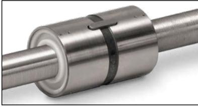
Capable of handling heavy loads, planetary roller screws contain precision ground rollers engaged with a precision ground screw and nut. When compared with a ball screw of the same size and lead, the roller screw components are designed to increase points of contact and a larger contact radius. This results in less stress per point of contact and allows roller screws to carry higher loads.
