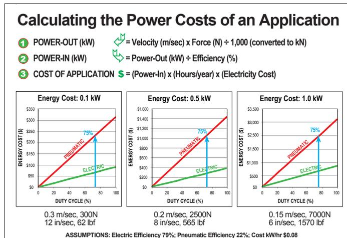
Figure 1: Calculating the power costs of an application
