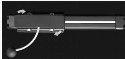
The second illustration shows what happens when the cylinder reaches one end of its stroke. When the carrier stops, inertia keeps the load moving forward, creating a dynamic twisting moment ( $M_z$ ) on the cylinder.
