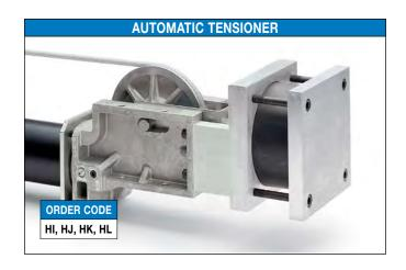
Automatic tensioners are required when a cylinder's stroke length is beyond the maximum stroke length for full manual cable adjustment for that bore size. The AT unit keeps the cable rigid and ensures maximum service life of both the cable and gland seals. AT units are also recommended for vertical lifting or severe, high-cyclic applications.
