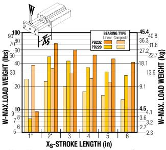
\*PB220, PB232 and PB252 - 1" Stroke and PB252 - 2" Stroke are units with one set of bearings.
