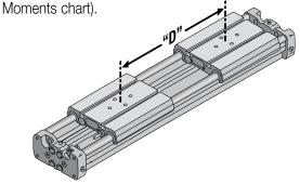
Determine your working stroke and your "D" dimension, then enter these into your configuration string. (Example: LS10SK30.00DW8.00RT2) The configurator will calculate the overall length of the actuator. Refer to page LS\_16 for complete LS ordering information.
