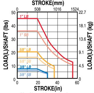
SB = Sintered Bronze Bearings LB = Linear Ball Bearings
