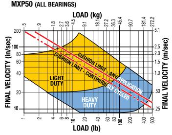
NOTE: If final (impact) velocity cannot be calculated directly, a reasonable guideline to use is 2X average velocity.
