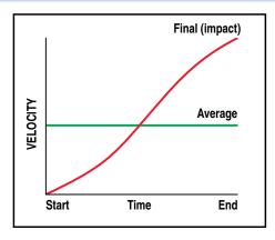
final (or impact) velocity. Rodless cylinders accelerate and decelerate at each end of the stroke. Therefore this acceleration must be considered (see diagram).
