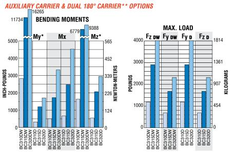
\*Auxiliary carrier bending moments indicated are at minimum center to center distance. Additional My + Mz load capacity can be obtained by increasing "D" dimension. Refer to auxiliary carrier data on page BC3\_5.
