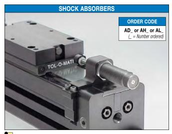
Rodless cylinders with standard internal cushion offer an effective method of decelerating loads. However, all Tolomatic rodless cylinders are capable of carrying heavier loads at higher velocities than the cylinder cushion can absorb. Optional shock absorbers can be used to increase the cylinder's life and broaden the application range for the cylinder model you have chosen.
