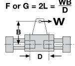
L should be below curve for the corresponding slide on the "Load vs. Stroke" chart (for sintered bronze or linear bearings - Mag Coupled Slides).
