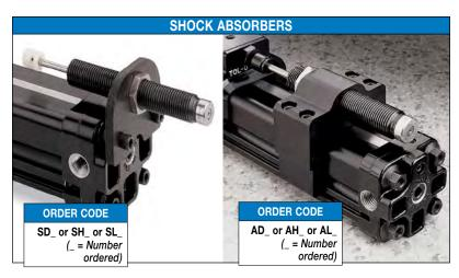
Rodless cylinders with standard internal cushion offer an effective method of decelerating loads. However, all Tolomatic rodless cylinders are capable of carrying heavier loads at higher velocities than the cylinder cushion can absorb. Optional shock absorbers can be used to increase the cylinder's life and broaden the application range for the cylinder model you have chosen.
