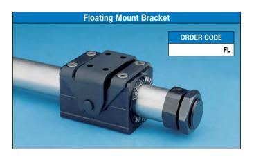
The integral floating mount bracket is available for applications in which a load is externally guided and supported and there is a need to compensate for non-parallelism between the cylinder and the independently-guided load.
