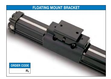
For applications where a BC2 band cylinder is moving a load that is externally guided and supported. An externally guided load, not parallel to the BC2 band cylinder may result in cylinder binding. The floating mount bracket compensates for nonparallelism between the cylinder and the external guide.
