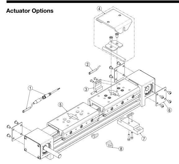
**To order service parts switches:** Switches for MXB include retained mounting hardware and are the same for all actuator sizes and bearing styles
