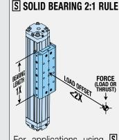
For applications using Solid bearings, binding or interrupted motion may occur if the load offset is equal to or greater than twice the bearing length (1X). LOAD OFFSET is defined as: the distance from the applied force (or the load center of gravity) to the centerline of the carrier.
