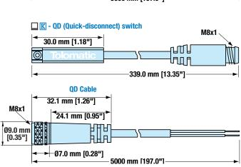
Dimensions in inches [brackets indicate dimensions in millimeters]
