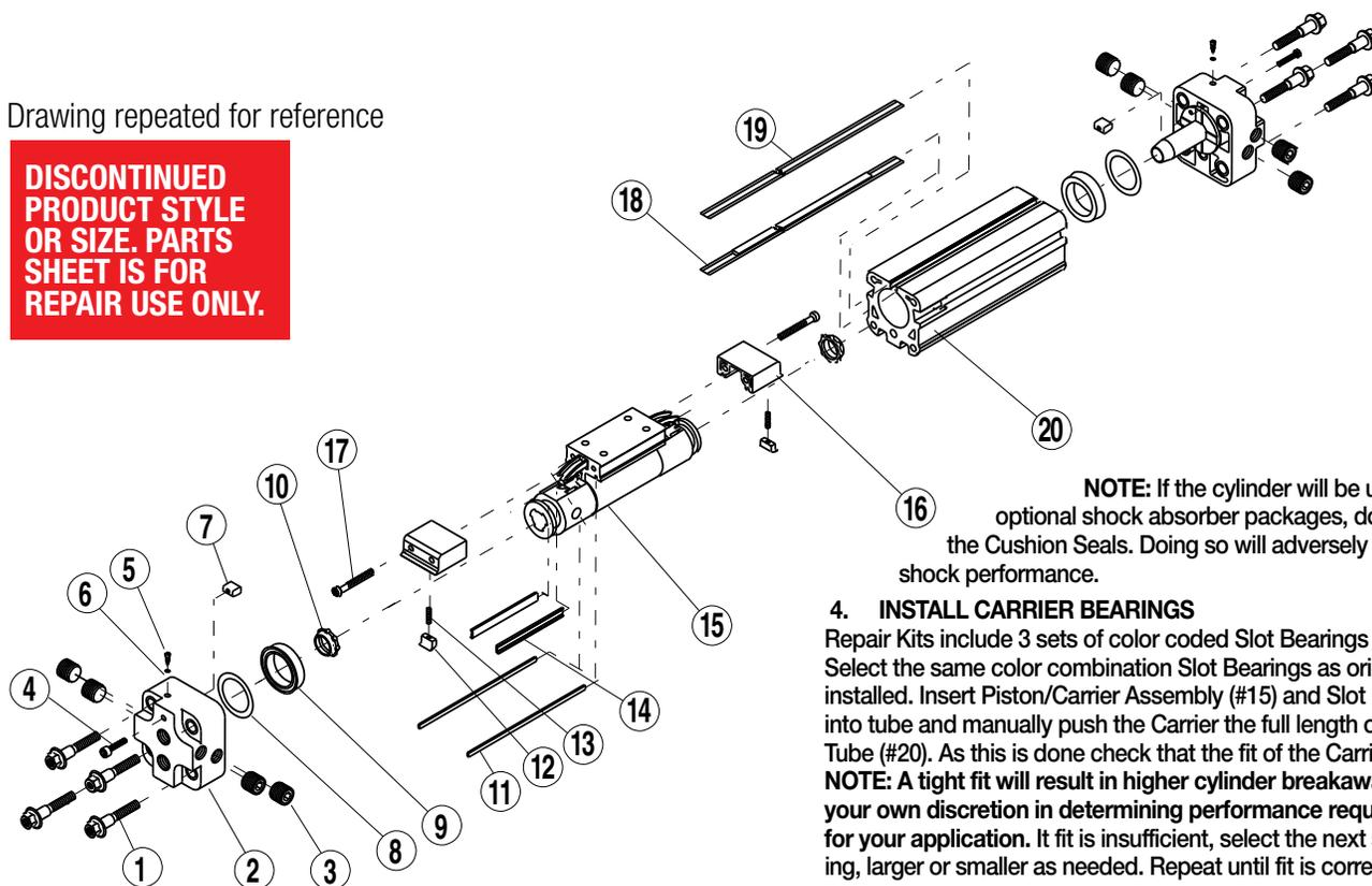
**NOTE:** If the cylinder will be used with optional shock absorber packages, do not install the Cushion Seals. Doing so will adversely affect shock performance.
