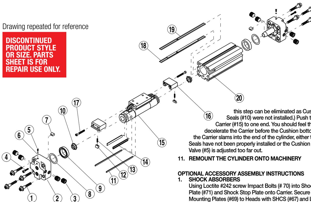
this step can be eliminated as Cushion Seals (#10) were not installed.) Push the Carrier (#15) to one end. You should feel the Cushion decelerate the Carrier before the Cushion bottoms out. If the Carrier slams into the end of the cylinder, either the Cushion Seals have not been properly installed or the Cushion Needle Valve (#5) is adjusted too far out.
