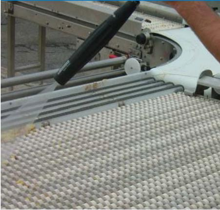
Cleaning a section of the high speed pizza conveying machinery near the waste removal door powered by the B3W10.
