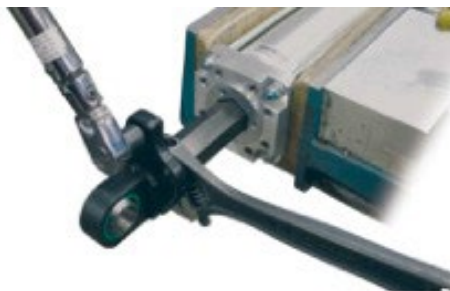
Figure 4.4: For Hex rod, hold thrust rod stationary using a wrench on the flat of the rod when attaching accessories, linkages or load to the actuator. Use a torque wrench to tighten the interfacing rod end to the actuator threaded connection point. Torque values provided in Table 4.1
