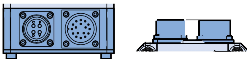
Figure 5.3: Drawing of box mount connectors used on some ServoWeld actuators.
