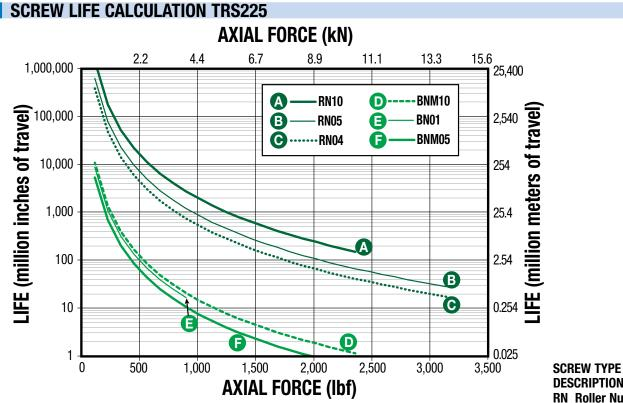
\*\*Life indicates theoretical maximum life of screw only, under ideal conditions and does not indicate expected life of actuator.
