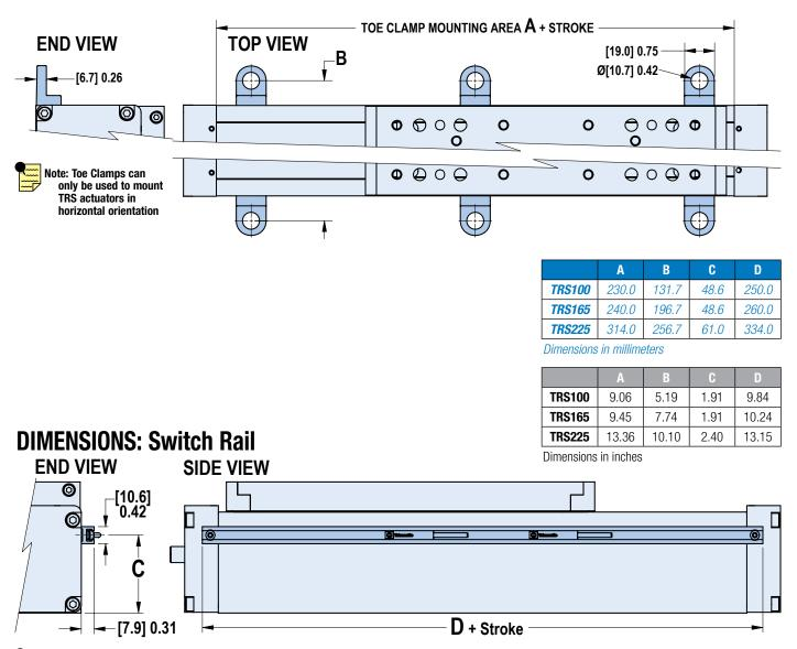
Note: Switch rail is installed on the right side of the actuator (from the motor end) for all motor mounting configurations except RPR1 where it is installed on the left side of the actuator.
