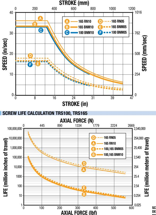
SCREW TYPE DESCRIPTION RN Roller Nut BN Ball Nut
