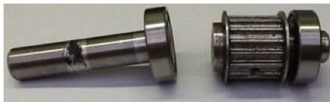
**Failed actuator driveshaft due to alignment/flex issues.**
