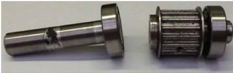
***Failed actuator driveshaft due to alignment/flex issues.***
