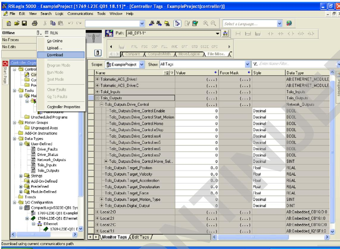
**Figure 24: Manipulating Data Tags in Controller Tags Window**
