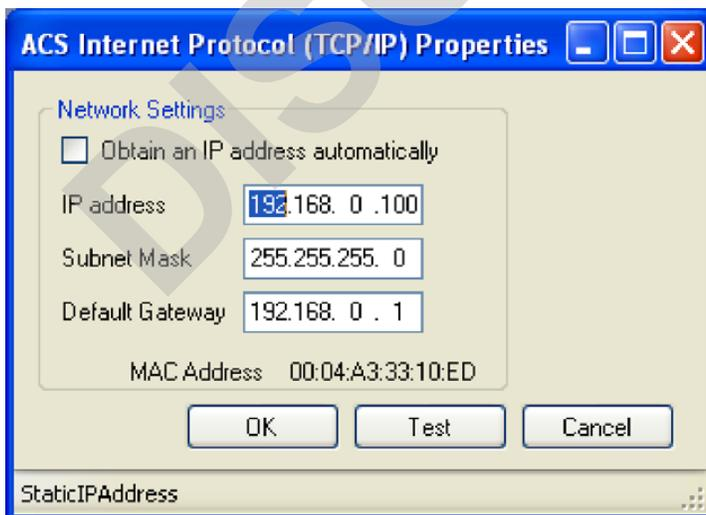
**Figure 1: Assigning ACS Drive an IP Address.**
