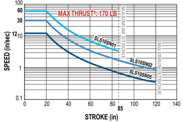
PV LIMITS: 12mm ACME METRIC SCREW w/25mm LEAD
