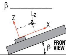
Load attached to carrier OR  Load supported by other mechanism
