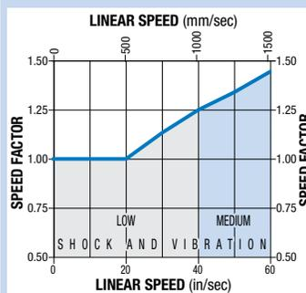
move. Speed should not exceed critical speed value as shown in graph (page SLS\_4-5) for the screw/nut combination chosen. Also, do not exceed safe rates of dynamic inertia moments determined in step #3.
