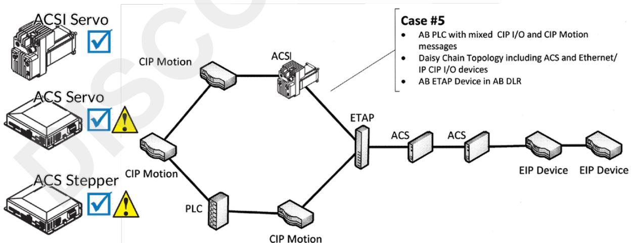
**CASE #5: PLC sending CIP Motion messages in Rockwell device level ring (DLR) with ACS drive connected with a 1783-ETAP device**
