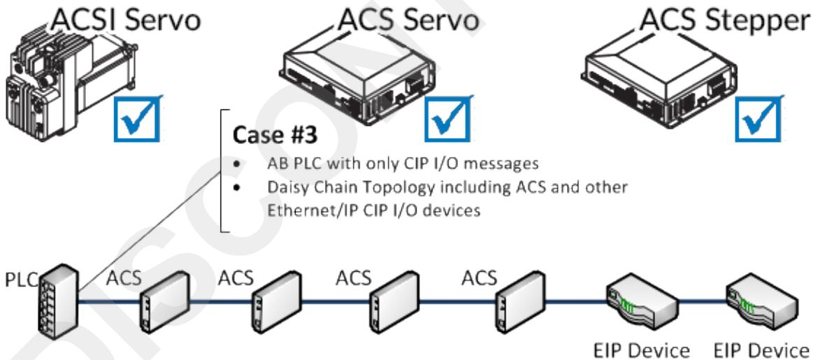
**CASE #3: PLC with only CIP I/O messages → daisy chain topology of ACS drives and other EtherNet/IP devices**
