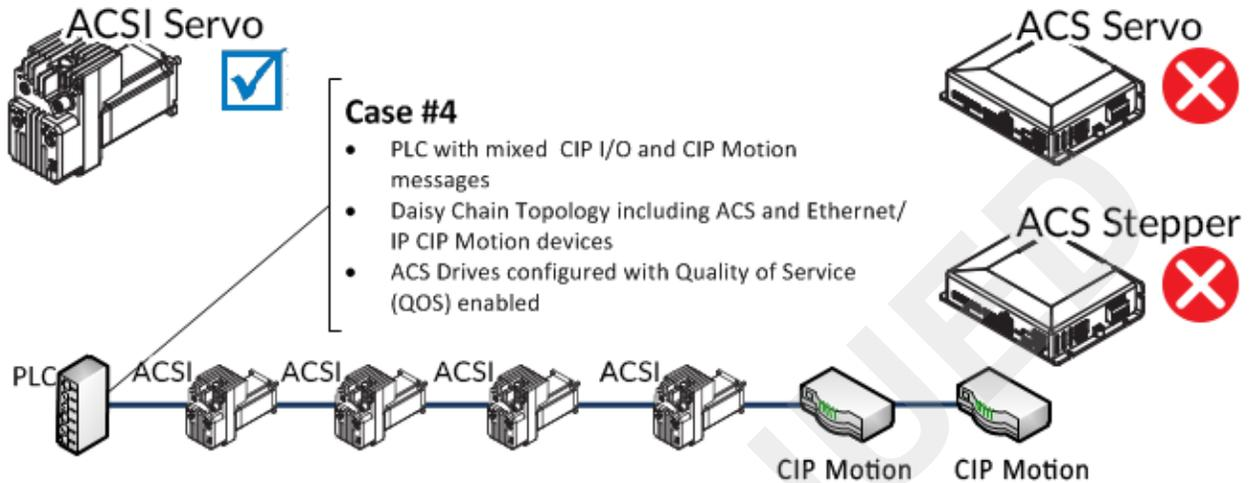
**CASE #4: PLC with CIP I/O and CIP Motion messages → daisy chain topology of ACS drives and other EtherNet/IP devices**
