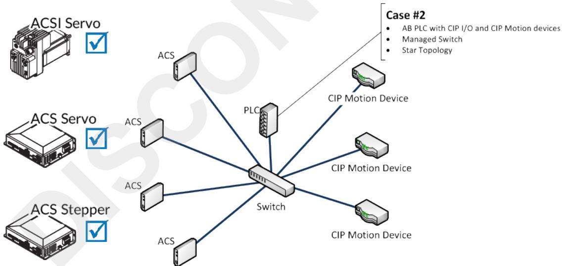
**CASE #2:** PLC with CIP I/O and CIP Motion messages → switch → star topology of ACS drives and other EtherNet/IP devices
