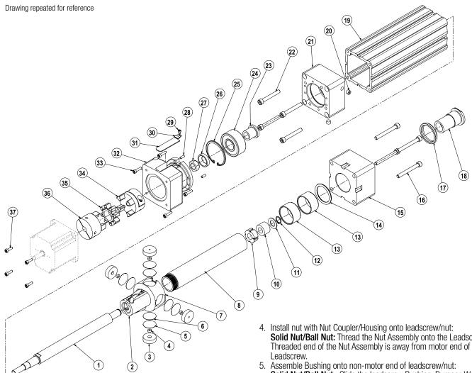
6. Remove Bearing from the Bearing Plate: Solid Nut/Ball Nut: Remove the Retaining Ring and press the Bearing out of the Bearing Plate as it is secured in place with retaining compound.
