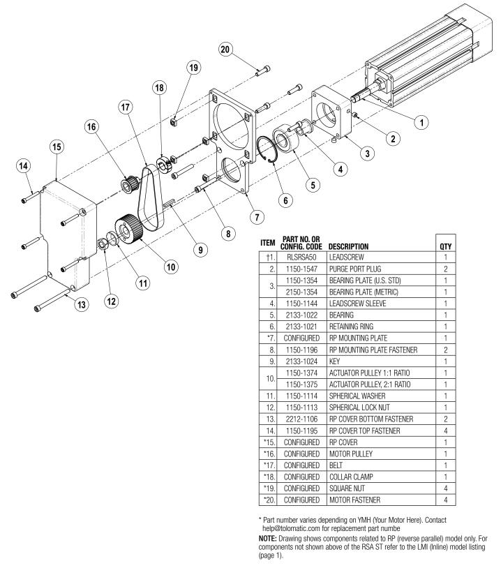
+ Replacement ordering method: RLS RSA50 \_\_\_\_ SK\_\_\_\_ ST NX
