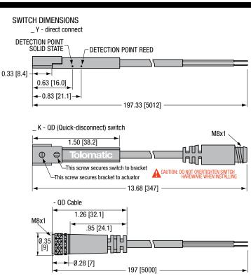
Dimensions in inches [brackets indicate dimensions in millimeters]
