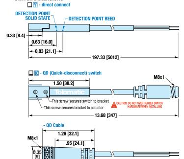
Dimensions in inches [brackets indicate dimensions in millimeters]
