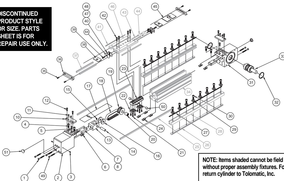
**NOTE: Items shaded cannot be field installed without proper assembly fixtures. For repair, return cylinder to Tolomatic, Inc.**
