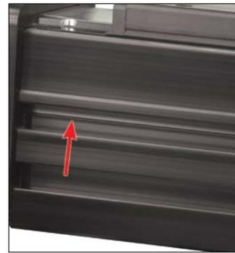
**⚠** THE NOTCHED GROOVE IN THE ACTUATOR INDICATES THE GROOVE TO INSTALL THE SWITCH. CONTACT TOLOMATIC IF SWITCHES ARE REQUIRED ON ANOTHER SIDE OF ACTUATOR.
