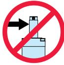
The IMA-S integrated motor actuator is not meant to be used in applications where side loading occurs. Loads must be guided and supported. Loads should be aligned with the line of motion of the thrust rod. Side loading will affect the life of the actuator.
