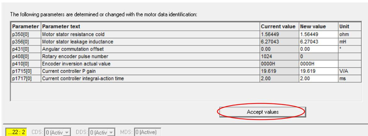
Stationary tuning is now complete. Adjusting the P-gain is the next step in tuning the actuator.
