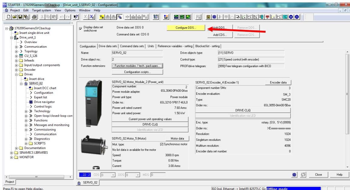
Under Function Modules select "Basic Positioner". Under Control Type, select "[21] Speed Control (with encoder)". After this click "next".
