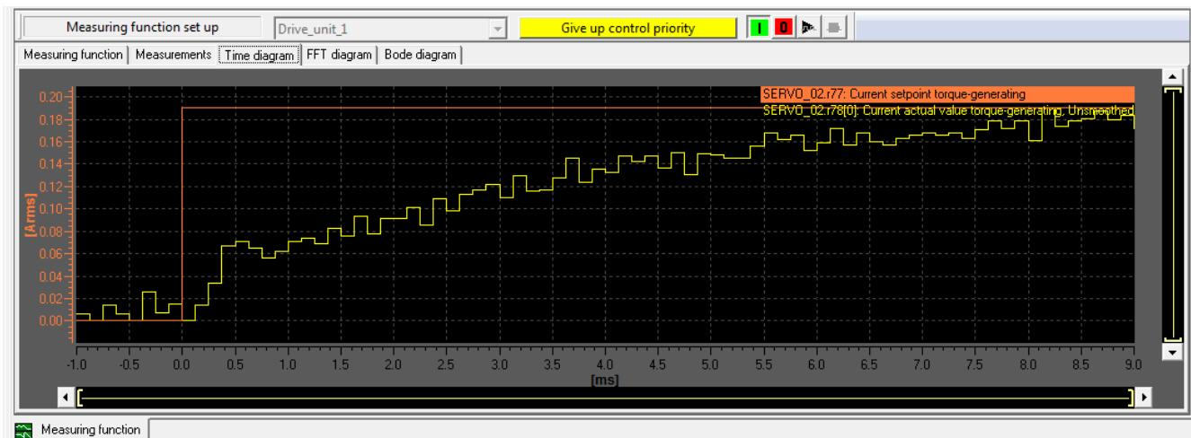
If the graph does not appear to match this graph, adjust the P gain in the motor menu until the measurement produces sufficient results.
