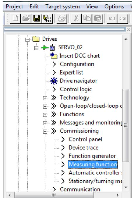
Next, under Measuring Function select: 'Current controller set point jump (after current setpoint filter)'
