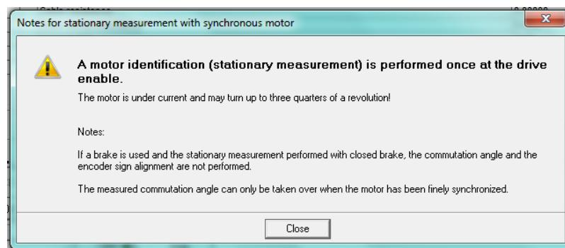
Turn the drive on by clicking the green box to perform the measurement. The drive will automatically power down after completing the measurement, this should take <5 seconds.
