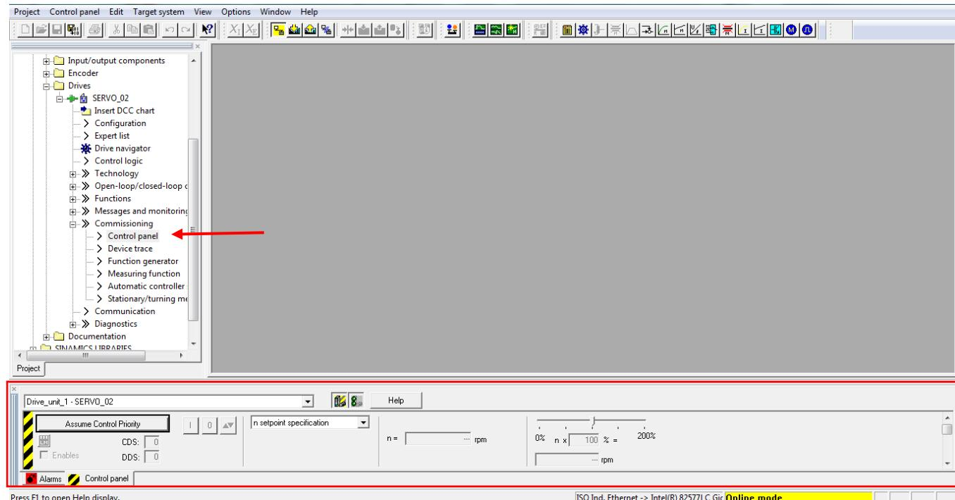
Under Commissioning, open the control panel and navigate to the 'Stationary/tuning measurement' tab.
