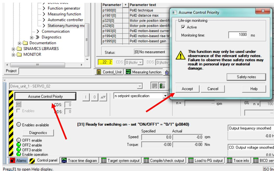
Check 'Enables' and turn the drive on by pressing the green 'I' box to perform measurement. The drive will momentarily turn on to initiate the measurement.
