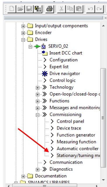
Then, select 'Stationary measurement' in the drop down.
