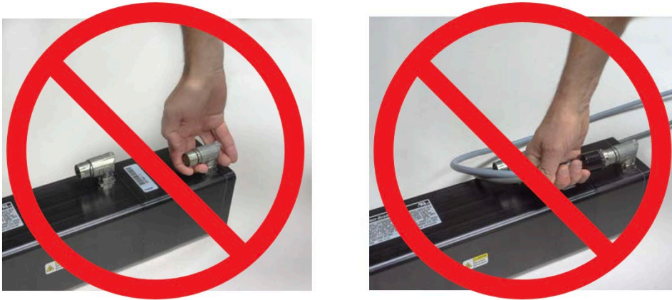
Figure 4.3: Do not carry IMA by connectors or cables.
