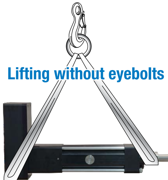
Figure 4-2 Lift RSX properly without eyebolts
