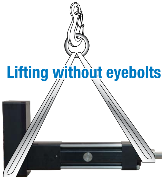
Figure 4-2 Lift RSX properly without eyebolts
