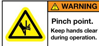
When installed, pinch points are generated capable of damaging forces. The risk area surrounding the actuator must either be guarded or clearly marked, including display signage in accordance with all applicable national and international legal requirements. The risk area must be protected by a safety system that stops the equipment if anyone enters the risk area. Personnel who enter the risk area must be authorized, trained and qualified for the different tasks inside the risk area.
