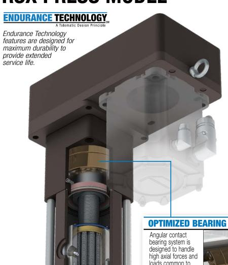
The RSX23P & RSX33P press actuators expand the compression force capability to 23 & 33 tons (46,000 & 66,000 lbf) making them well suited for applications such as pressing, riveting, clinching and many others. These press models have the same features as the standard RSX on pages 4 & 5 plus oversized tie rods, a bearing system optimized for high force extend, and a high strength steel front flange.
