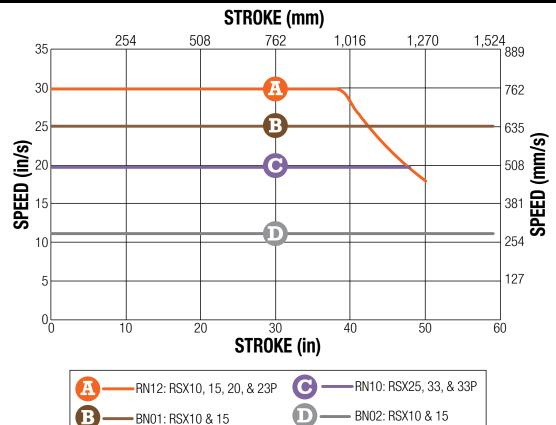
\*NOTE: When using Trunnion Mount, (TRR) consider the stroke to be longer when determining Critical Speed and Buckling Load:
