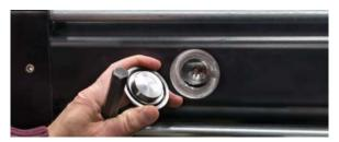
Remove the access cover, and extend or retract the thrust rod for access to the internal grease zerk.
