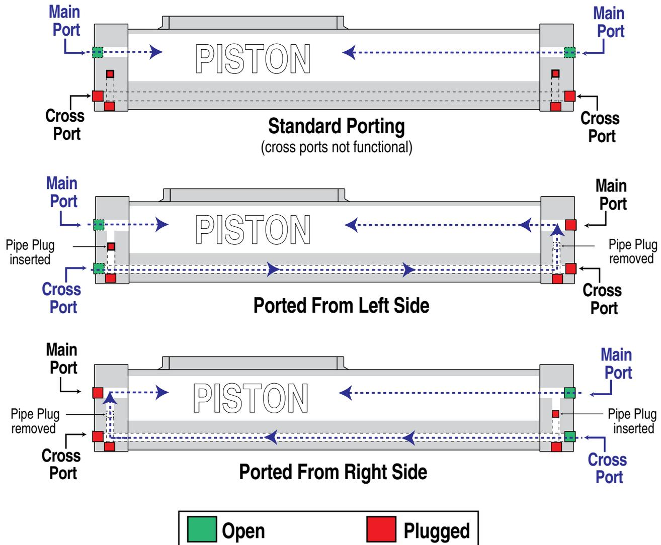
NOTE: Standard porting may be field converted to ported from left or ported from right. For complete instructions refer to parts sheet.
