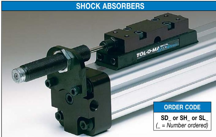
Rodless cylinders with standard internal cushion offer an effective method of decelerating loads. However, all Tolomatic rodless cylinders are capable of carrying heavier loads at higher velocities than the cylinder cushion can absorb. Optional shock absorbers can be used to increase the cylinder's life and broaden the application range for the cylinder model you have chosen.
