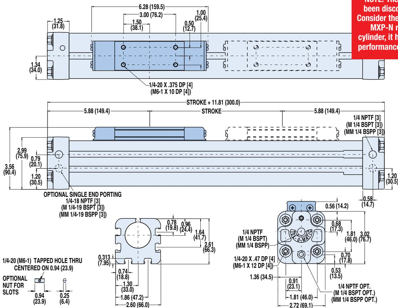
Dimensions in inches (parenthesis indicate dimensions in millimeters)
