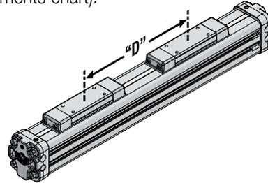
Determine your working stroke and your "D" dimension, then enter these into your configuration string. (Example: BC415SK50.00DW15.00RT2) The configurator will calculate the overall length of the actuator.
