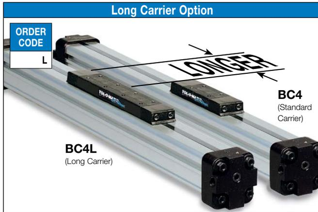
**Long carrier option greatly increases the “My” and “Mz” moment load capacity.** This broadens the application range for these models. Other benefits include larger mounting surface and virtual elimination of chatter for vertical cantilever loads.
