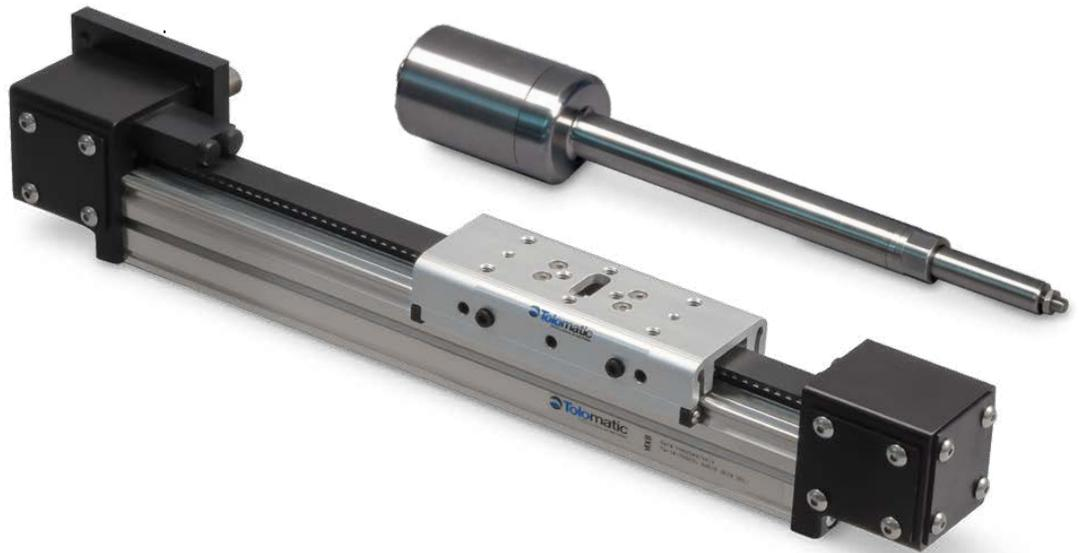
Above are examples two different actuator types: Rod-style and rodless. The inherent sealing properties of the rod-style actuator make it the only logical choice for wash-down environments where actuator shielding is not possible.
