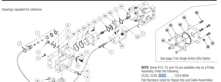
are for standard cylinders only. Always make reference to the complete configuration Number on your cylinder when ordering replacement items, also specify the stroke length.
