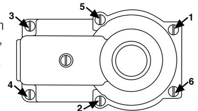
**Lubrication:** All Float-A-Shaft® gear boxes have been lubricated at the factory with Mobilith® SHC 460. However, units require more lubrication prior to operation. Periodic re-lubrication is also necessary for optimum performance. When re-lubricating, inject Mobilith® SHC 460 (maximum operating temperature of 300°F or higher and EP rated) into gear case, as required, via the grease zerk provided. Mobilith® SHC 460 - 14 oz grease cartridge • P/N 0100-1605
