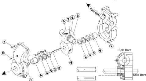
Thrust Washer (2), and the other Flanged Bushing (6). Position this assembly into the Gear Case Housing (1), making sure the teeth of the gears mesh.
