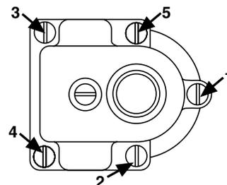
**Lubrication:** All Float-A-Shaft® gear boxes have been lubricated at the factory with Mobilith® SHC 460. However, units require more lubrication prior to operation. Periodic re-lubrication is also necessary for optimum performance. When re-lubricating, inject Mobilith® SHC 460 (maximum operating temperature of 300°F or higher and EP rated) into gear case, as required, via the grease zerk provided. Mobilith® SHC 460 - 14 oz grease cartridge • P/N 0100-1605
