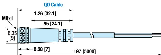
Dimensions in inches [brackets indicate dimensions in millimeters]
