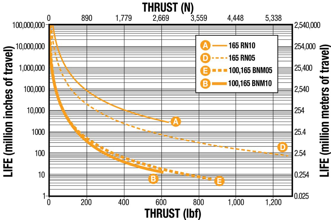
\*Life indicates theoretical maximum life of screw only, under ideal conditions and does not indicate expected life of actuator.
