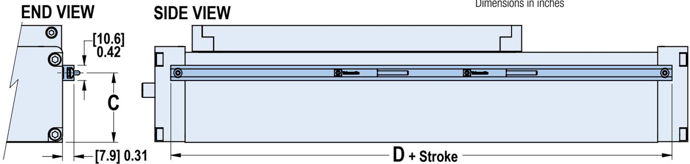
Note: Switch rail is installed on the right side of the actuator (from the motor end) for all motor mounting configurations except RPR1 where it is installed on the left side of the actuator.
