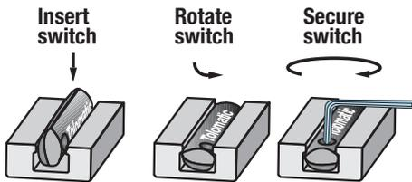
Place switch in side groove on tube at desired location with "Tolomatic" facing outward. While applying light pressure to the switch, rotate the switch halfway into the groove. Maintaining light pressure, rotate the switch in the opposite direction until it is fully inside the groove with "Tolomatic" visible. Re-position the switch to the exact location and lock the switch securely into place by tightening the screw on the switch.
