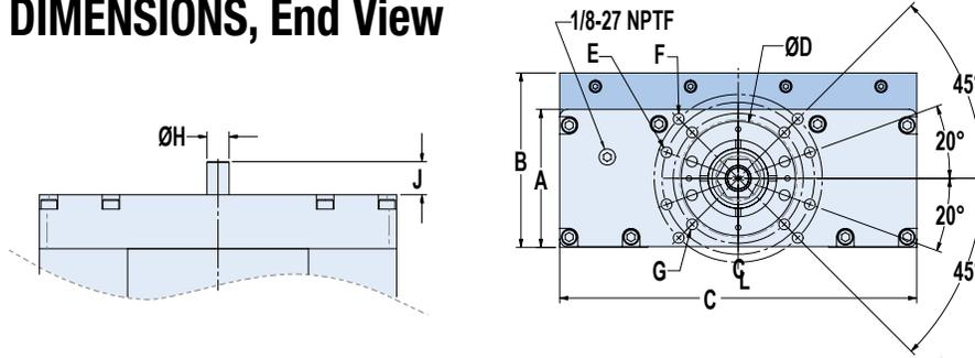
**No Motor Mount** (threaded holes and bolt circle; *when no motor mount is selected*)
