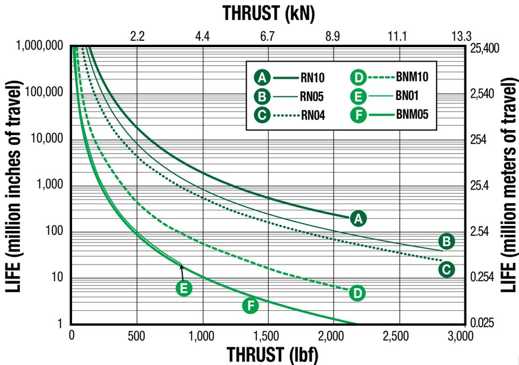
\*\*Life indicates theoretical maximum life of screw only, under ideal conditions and does not indicate expected life of actuator.
