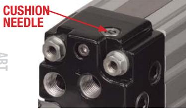
zero. If the carrier reaches the end of stroke at velocity, then the cushion needs to be increased by turning the cushion needle screw clockwise. If the carrier stalls or bounces (quickly oscillating directions) before it reaches the end of stroke, then the cushion needs to be decreased by turning the cushion needle screw counterclockwise. Improper cushion adjustment may cause premature failure of the actuator. Call Tolomatic with any questions.
